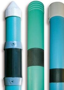
PVC Durvinil® grouting pipes used to perform injections of cement mixtures and resins as part of interventions of soil consolidation and waterproofing; they are also essentials in the excavation of tunnels, construction of dams, reinforcement of foundations.
